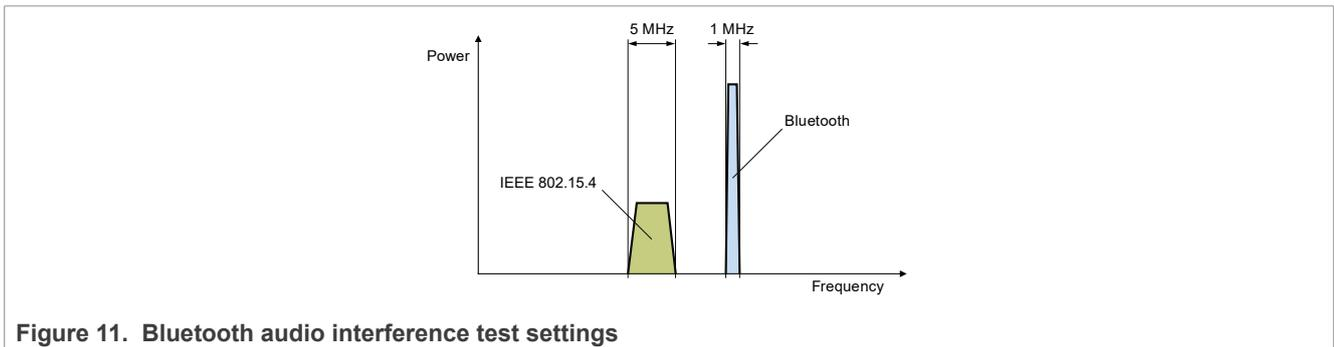
Figure 11. Bluetooth audio interference test settings
