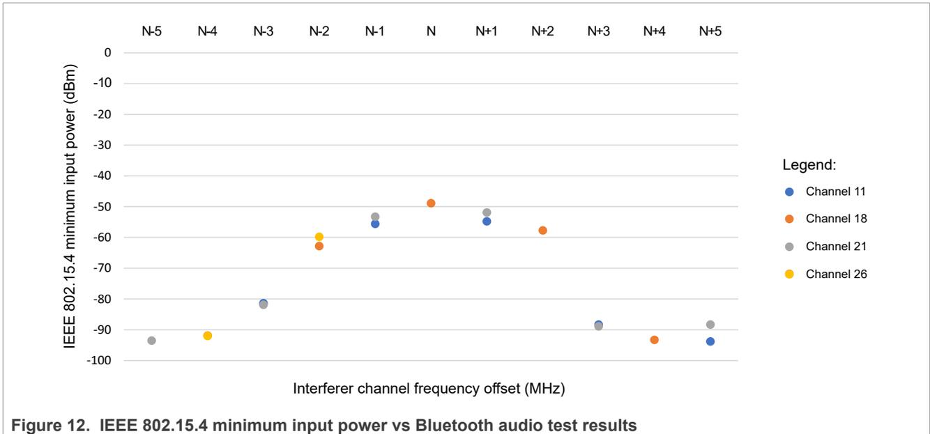
Figure 12. IEEE 802.15.4 minimum input power vs Bluetooth audio test results
