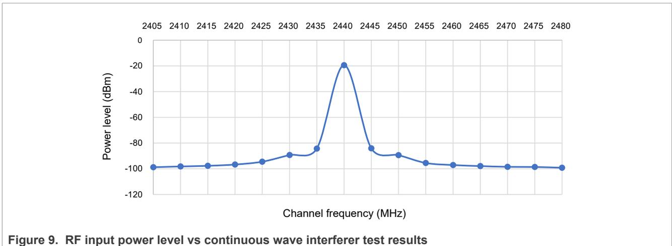
Figure 9. RF input power level vs continuous wave interferer test results
