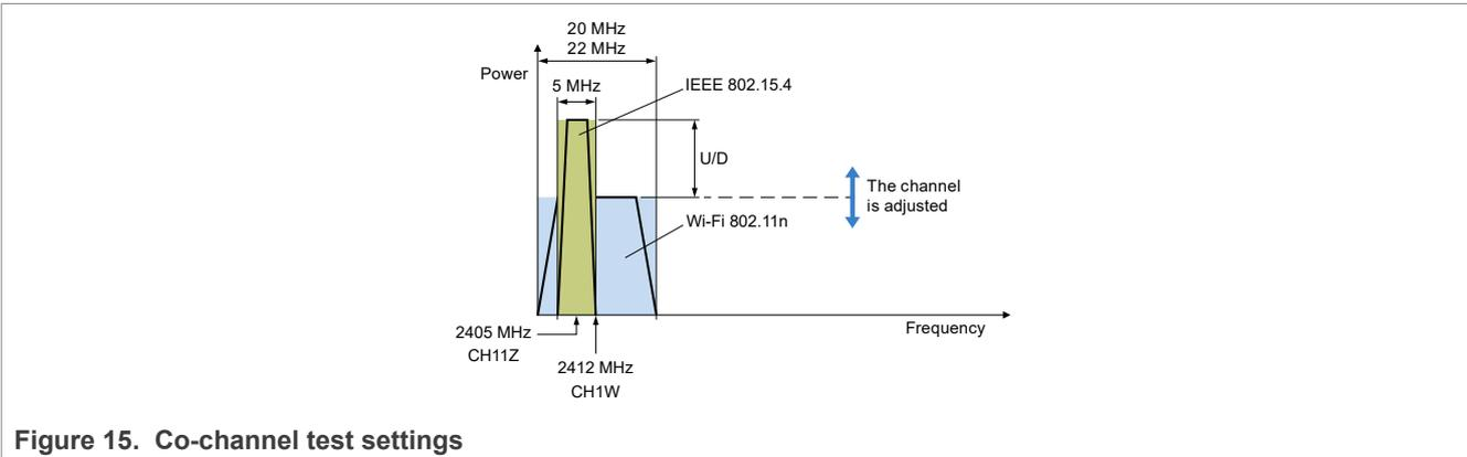
5.2 Wi-Fi interference tests
