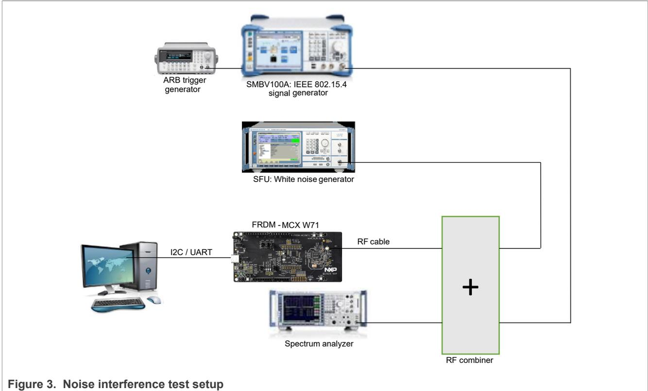
Figure 3. Noise interference test setup
