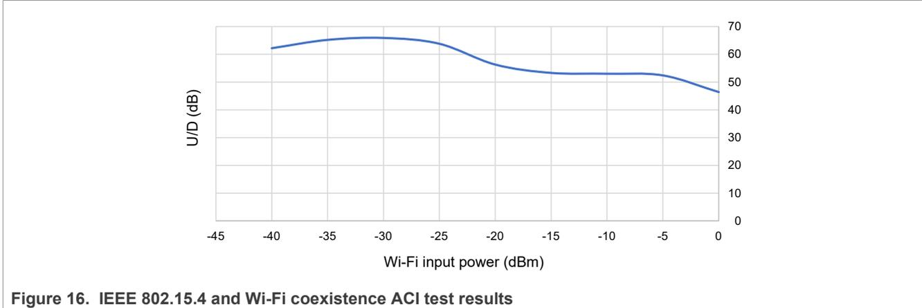
Figure 16. IEEE 802.15.4 and Wi-Fi coexistence ACI test results
