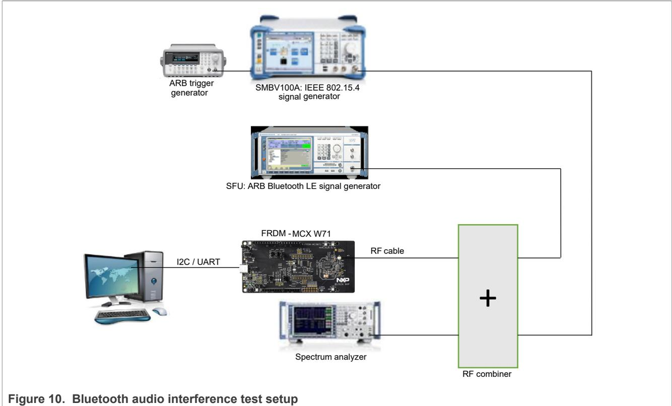
Figure 10. Bluetooth audio interference test setup
