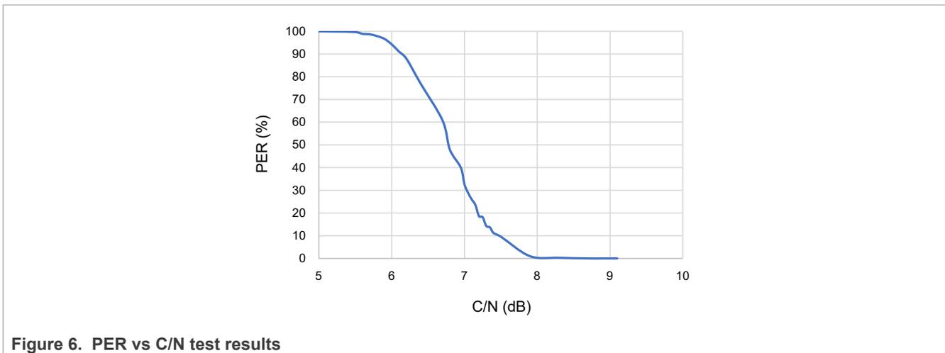
Figure 6. PER vs C/N test results
