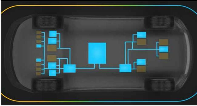
The new generation of CAN partial networking transceivers is introduced in combination with two technologies: CAN FD on TJA144x, and CAN FD with Signal Improvement Capabilities (CAN SIC) on the TJA146x, which supports use cases where higher CAN speeds up to 8 Mbit/sec and/or highly complex topologies are targeted.
