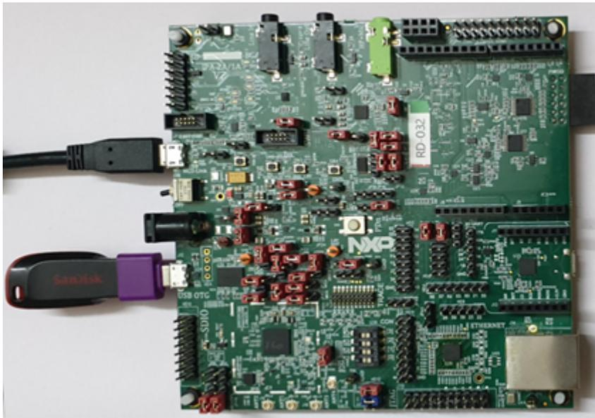
Figure 1. USB drive plugged into RW61x EVK board
