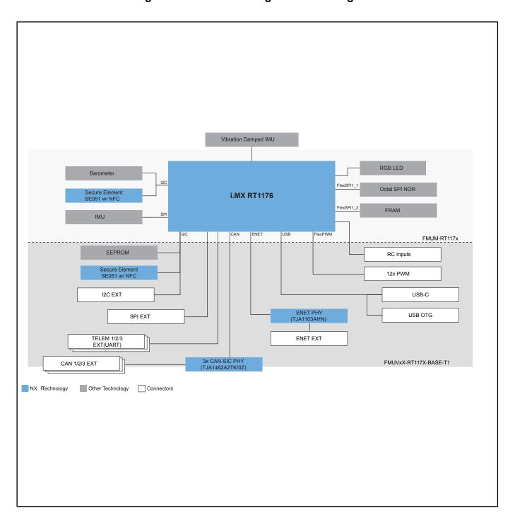
**Drone System Block Diagram Block Diagram**
